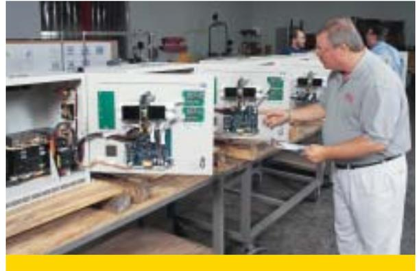
Simulator for on-site product testing. The accepted standard for sustained product life evaluation, the KeyTek ECAT permits on-site testing with amperages of up to 10,000 amps and voltages as high as 20,000 volts. SElect suppression filter systems are subjected to strenuous testing and inspection by diligent quality assurance professionals before leaving the factory, and every unit is shipped with a Diagnostic Signature Card listing factory-established benchmark performance values.\*
